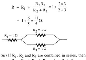
(*iii*) If  $R_1$ ,  $R_2$  and  $R_3$  are combined in series, then  $R = R_1 + R_2 + R_3 = 1 + 2 + 3$   $= 6\Omega$
