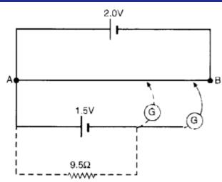
1.5 V cell. The balance point of the cell in open circuit is 76.3 cm. When a resistor of 9.5  $\Omega$  is used in the external circuit of the cell, the balance point shifts to 64.8 cm length of the potentiometer wire. Determine the internal resistance of the cell. **Answer:**
