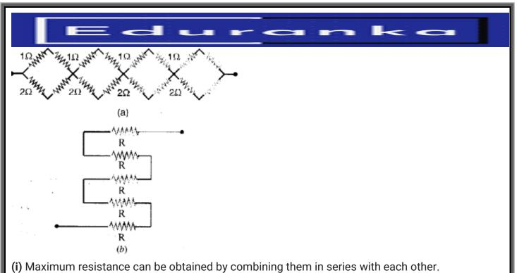
The maximum resistance  $R_{max} = R + R + R + ....n$  times = nR.
