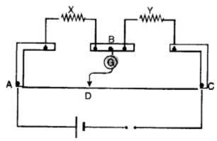
(b) Determine the balance point of the bridge above if X and Y are interchanged.(c) What happens if the galvanometer and cell are interchanged at the balance point of the bridge?
