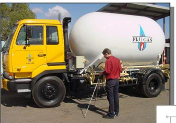
★ Road Tankers designed and built by Air & Gas Industries are tested for low noise in line with the requirements for external noise as specified in Australian Design Rule 28/01 and the Queensland Government Environmental Protection (Noise) Policy 2008.
