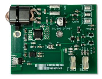
So we designed up a new driver board that replaces all 3 of the original MOSFETS. Our new board uses one LDMOS driver that is very much over qualified to handle the job. The system is a direct replacement and becomes the new driver for both the 2 Meter and HF/6M bands. And the tracking is amazing! You will notice that the power output signal levels track very closely with the settings in the menu on the radio.
