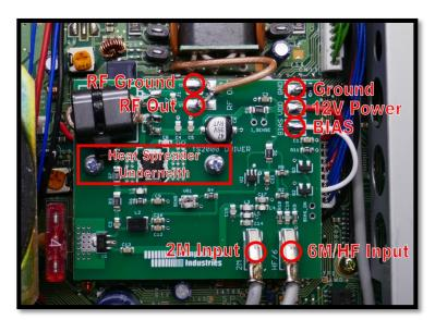
sometimes less. One thing we have noticed is that how you connect the coax output cable can affect 2 meters.
