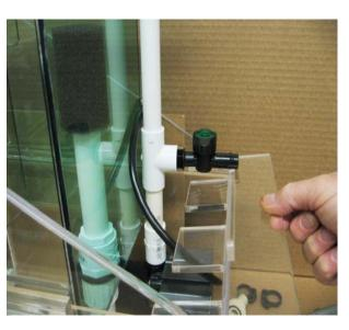
Slip 21/2" section of vinyl hose over lower valve then secure with hose clamp
