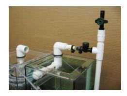
Install  $\frac{1}{2}$ " MPT x 16mm barbed control valve into lower manifold. Then install sump lid.
