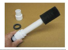
Install threaded end of the stand pipe assembly through bottom hole of the refugium tank.
