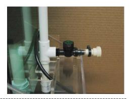
Prepare Venturi Protein Skimmer influent parts in numerical order. Insert 1<sup>st</sup> street elbow into intake facing upward, and the 2<sup>nd</sup> facing right.
