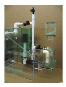
Assemble and install Effluent CPVC (Tan) plumbing from skimmer effluent to drain into wet dry filter sump. NOTE: Effluent parts are NOT pressurized so it may not be necessary to bond unless a problem arises.
