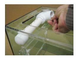
Insert threaded nipple through unit top and into spray bar elbow. Lightly tighten with putty knife.
