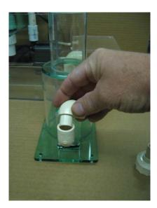
Install nut section of union. Be careful not to loose rubber seal inside.
