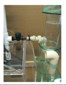
Secure Protein Skimmer to HO bracket using nylon screws and wing nuts.
