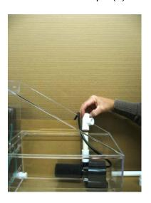
Insert 8¼" length section of ½" PVC Pipe (III) into ½" Tee (III)
