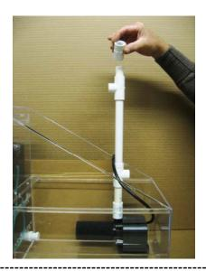
Thread ½" MPT control valves into tee & top adapter. Slip 2½" section of vinyl hose over valve then secure with hose clamp.
