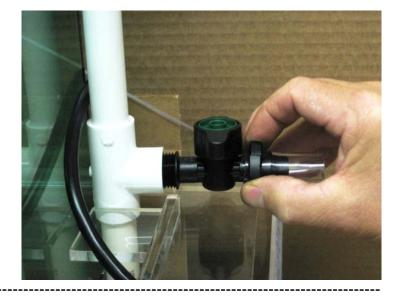
Insert threaded half union portion into ½" section of vinyl hose then secure with hose clamp
