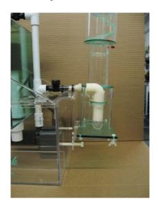
Twist nylon adjustment bolts to level and align Protein Skimmer. Secure protein skimmer influent line to manifold using a union fitting.
