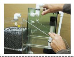
Slide vinyl hose from manifold valve over refugium intake fitting then secure using plastic hose clamps.
