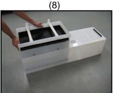
9. Insert the rigid air injection tubes through the front panel and into the bio-media. (wetting the tubes first eases installation)
