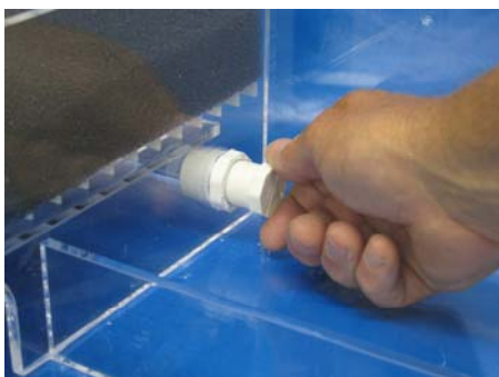
(8) Remove plug from filter wall.
