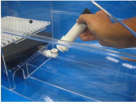
(11) Install stand pipe over elbow.
