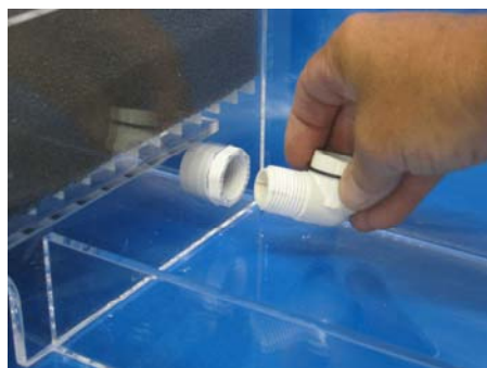
(9) Thread 90° elbow into bushing.
