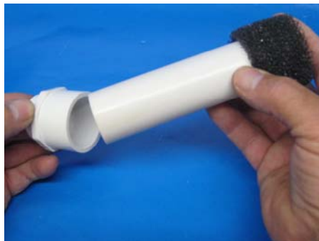
(7) Insert Stand pipe pressing completely into reducer fitting
