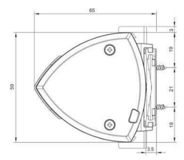
V1 can be easily installed on existing concealed sliding doors and com-plies with the EN16005 standard, "Low Energy Movement" section, that manages the door speed by a sophisticated electronic control with no need of sensors or safety photocells.
