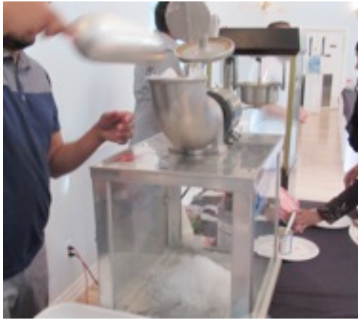
Add ice cubes to the top - press down top lid which crushes the ice cubes...
