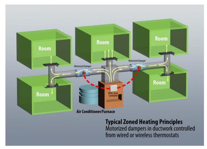
Zoned heating and cooling principles do not offer room-to-room climate control.
