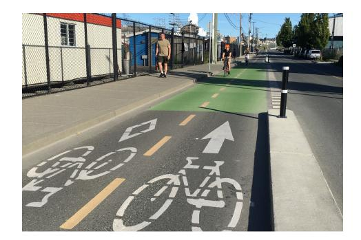
A bi-directional protected facility is when both bike lanes are on the same side of the street. In certain road and geometric contexts, bi-directional bike facilities are more suitable as they can take up less road space and preserve parking on one side of the road, for example. One of the main drawbacks with bidirectional facilities is that they can present more conflicts with motor vehicles turning.
