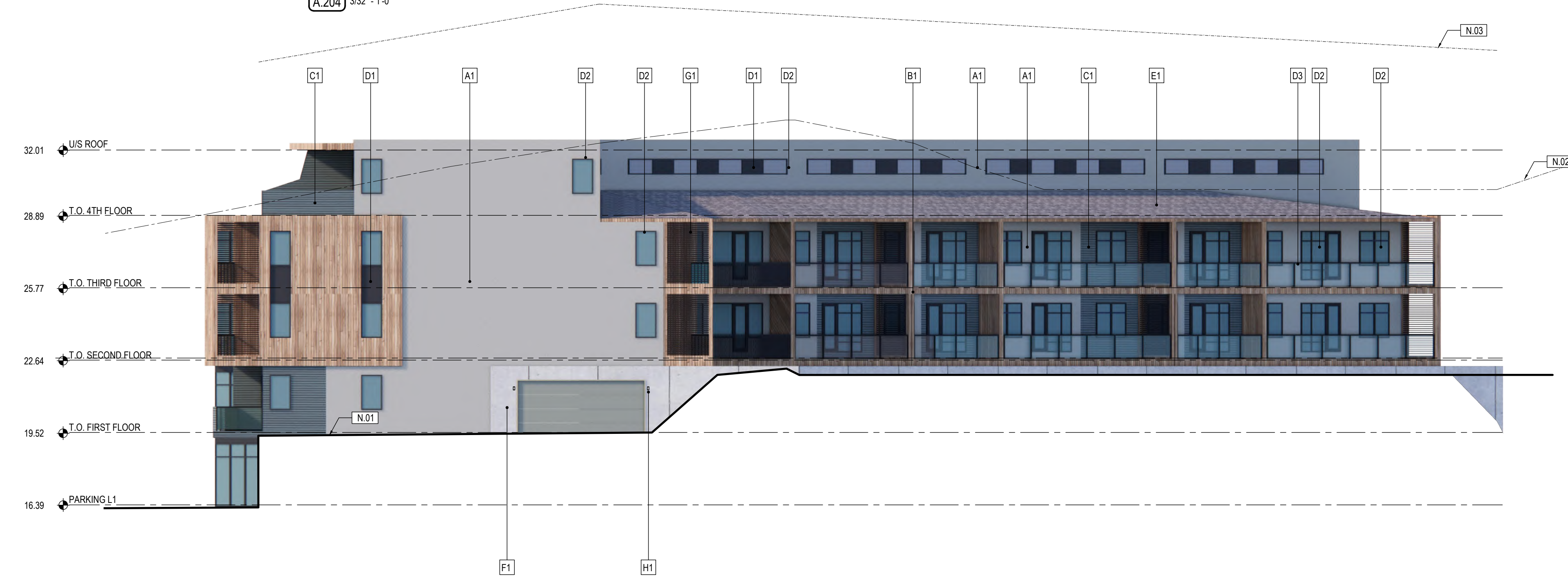
2 SOUTH WEST ELEVATION A.204 3/32" - 1'-0"
