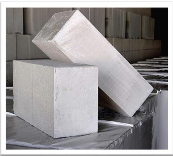
Figure 1: 12x8x24 AAC Block
