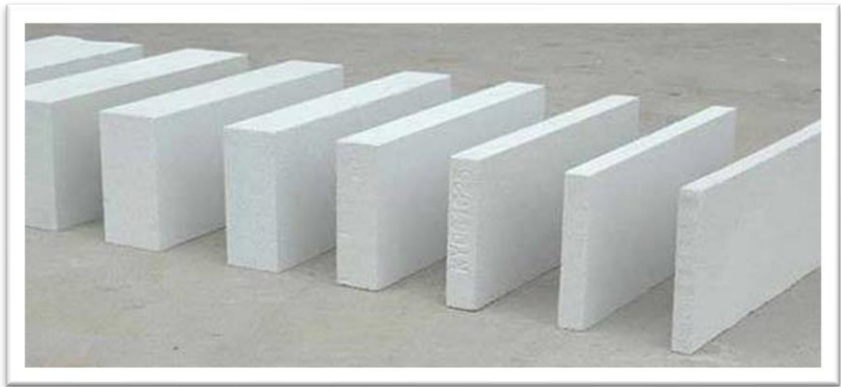
Figure 3: Different-Sized AAC Panels and Blocks
