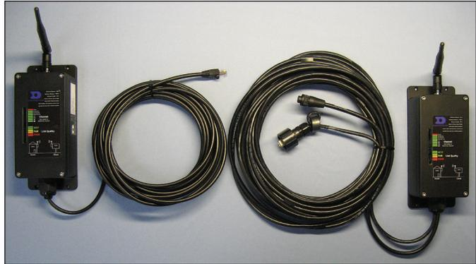
**Figure 1:** Ethernet Bridge Radios – Two-Wire Client Radio
