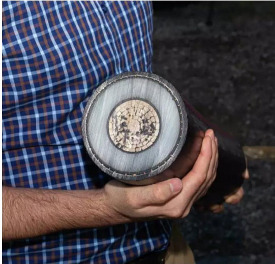
A cross-section of the 5-inch, direct-current transmission cable being laid underground and underwater as part of the 339-mile Champlain Hudson Power Express. Work on the project is ongoing throughout the Capital Region. Photo provided
