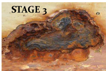
Stage 3 corrosion is found with heavy scale and minor edge erosion.
