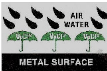
Cortec® VpCIs bond with metal surfaces to form a protective 'Molecular Umbrella,' sealing out air and moisture that cause rust and corrosion.
