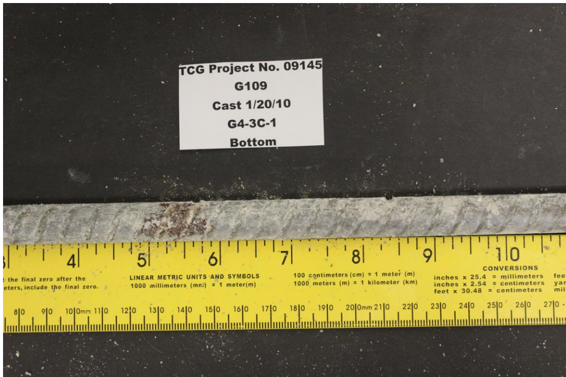
Figure 15 – Top Bar from 2005NS Beam, showing the bottom surface
