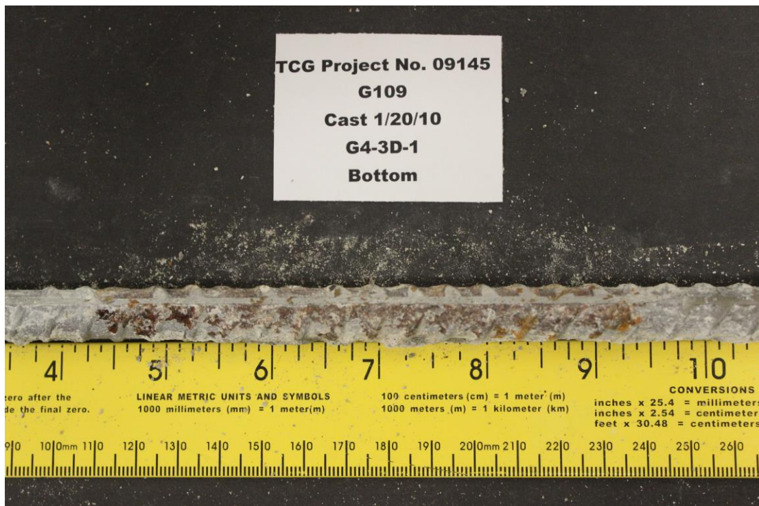
Figure 17 – Top Bar from 2005NS Beam, showing the bottom surface
