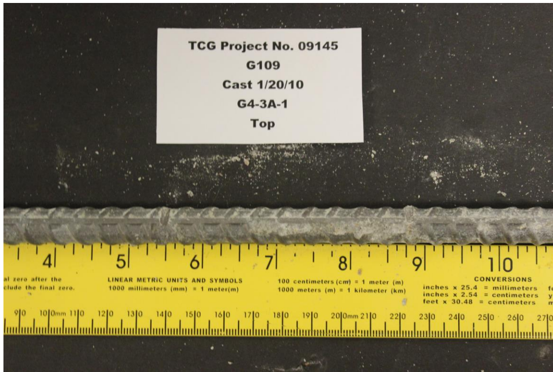
Figure 10 - Top Bar from 2005NS Beam, showing the top surface
