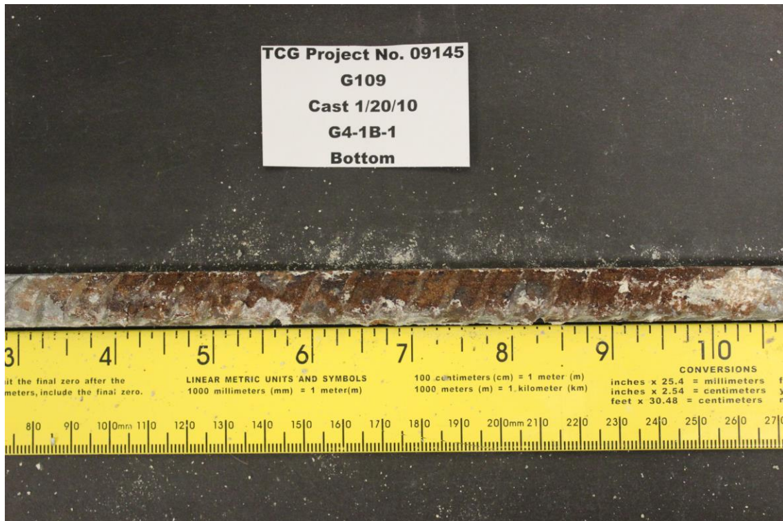
Figure 5 – Top Bar from Control Beam, showing the bottom surface
