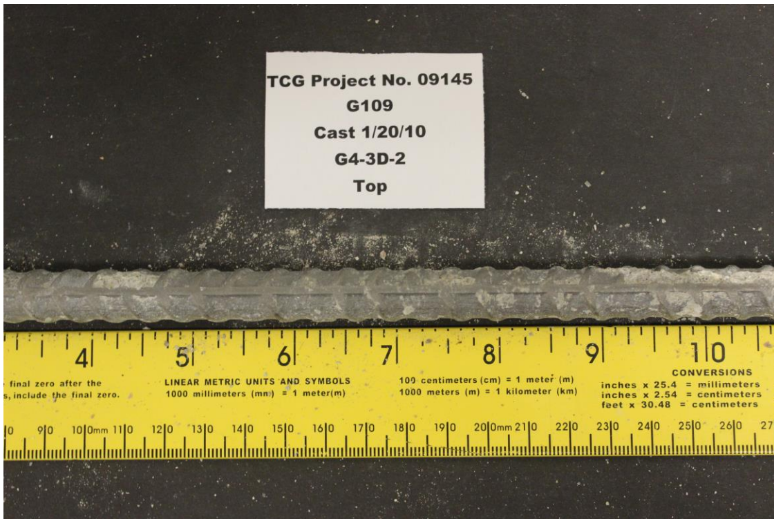
Figure 16 - Top Bar from 2005NS Beam, showing the top surface
