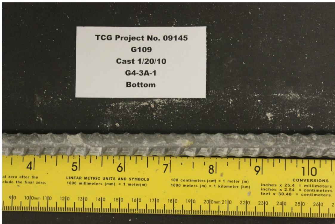
Figure 11 – Top Bar from 2005NS Beam, showing the bottom surface
