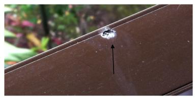
Additionally, the image seen where there is a perforation of the surface and the white particulate build up - that white build up is aluminum oxides - and is often confused with salt deposits.
