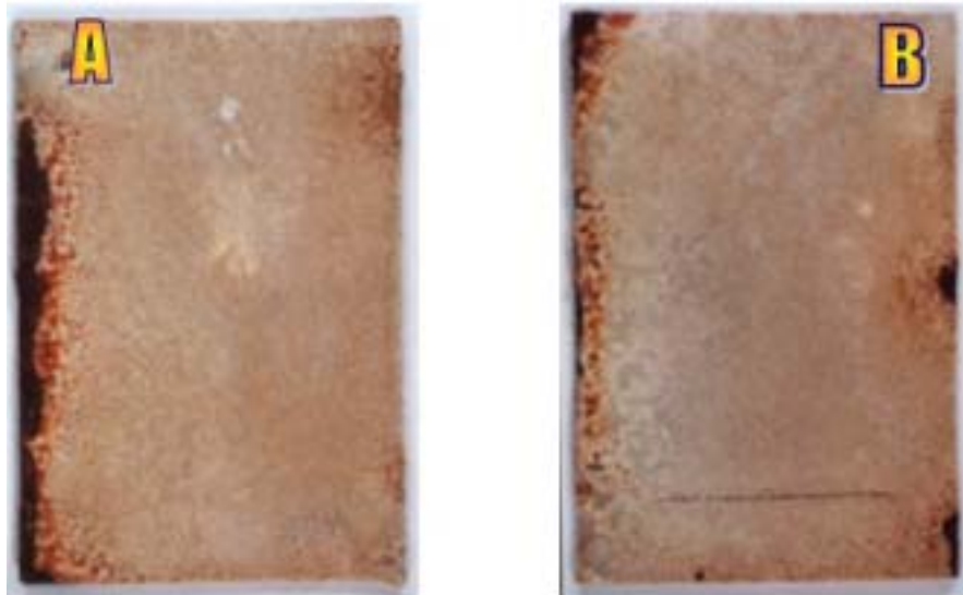
Galvanized steel: a) without incision, and b) with incision, after 42 months' exposure at La Voz Station.
