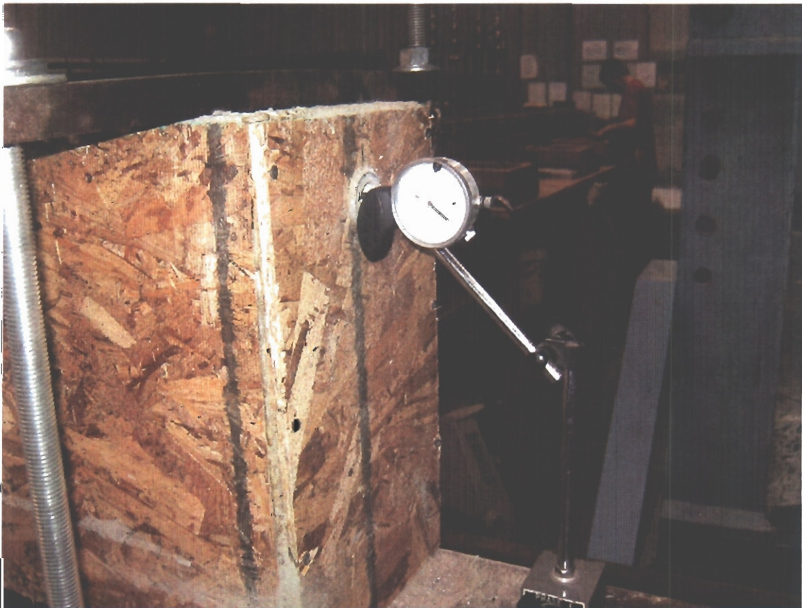
Photo 2: Dial indicator for elongation measurements
