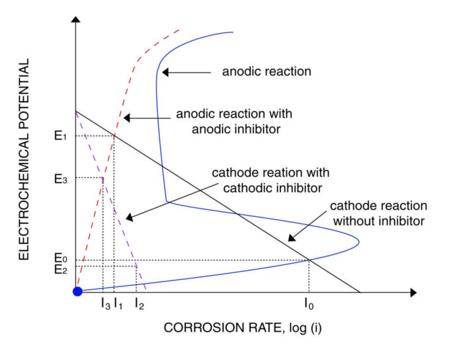
Fig. 1: The effect of inhibitors on corrosion potential and corrosion current density
