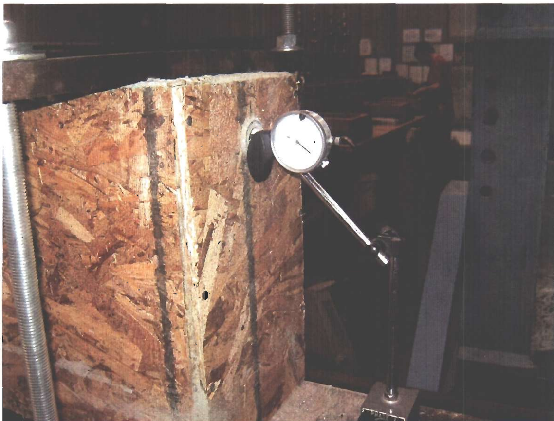
Photo 2: Dial indicator for elongation measurements
