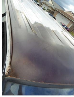
1<sup>st</sup> Coat Cortec Corrverter Dried to touch
