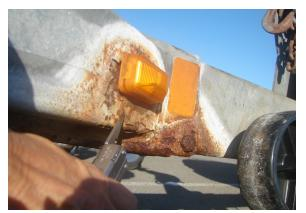
Once the scale is removed from select areas (best area to pull scale from is where the heaviest scale build up is found) is to put the sharp tip against the newly exposed metal. Move tip back about  $2^{"} - 3^{"}$  and then tap the tip against the heavy metal to remove the rusted scale. Be sure to hold the tool firmly as the impact may cause you to loose grip and possibly drop tool. (Don't perform this if your wearing slippers or tennis shoes! Your safety is paramount in any work you do.)
