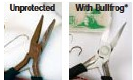
Two identical tackle boxes were placed inside a profession chamber that accelerates corrosion. After several weeks of continuous exposure to salt spray and temperature and humidity extremes the equipment with the Bullfrog® VpCI® protection still looks like new.
