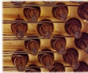
An older piano often will develop a lot of rust on the strings, especially in tropical or high humidity areas.
