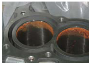
Standard Corrosion Protection Packaging: RUSTED
