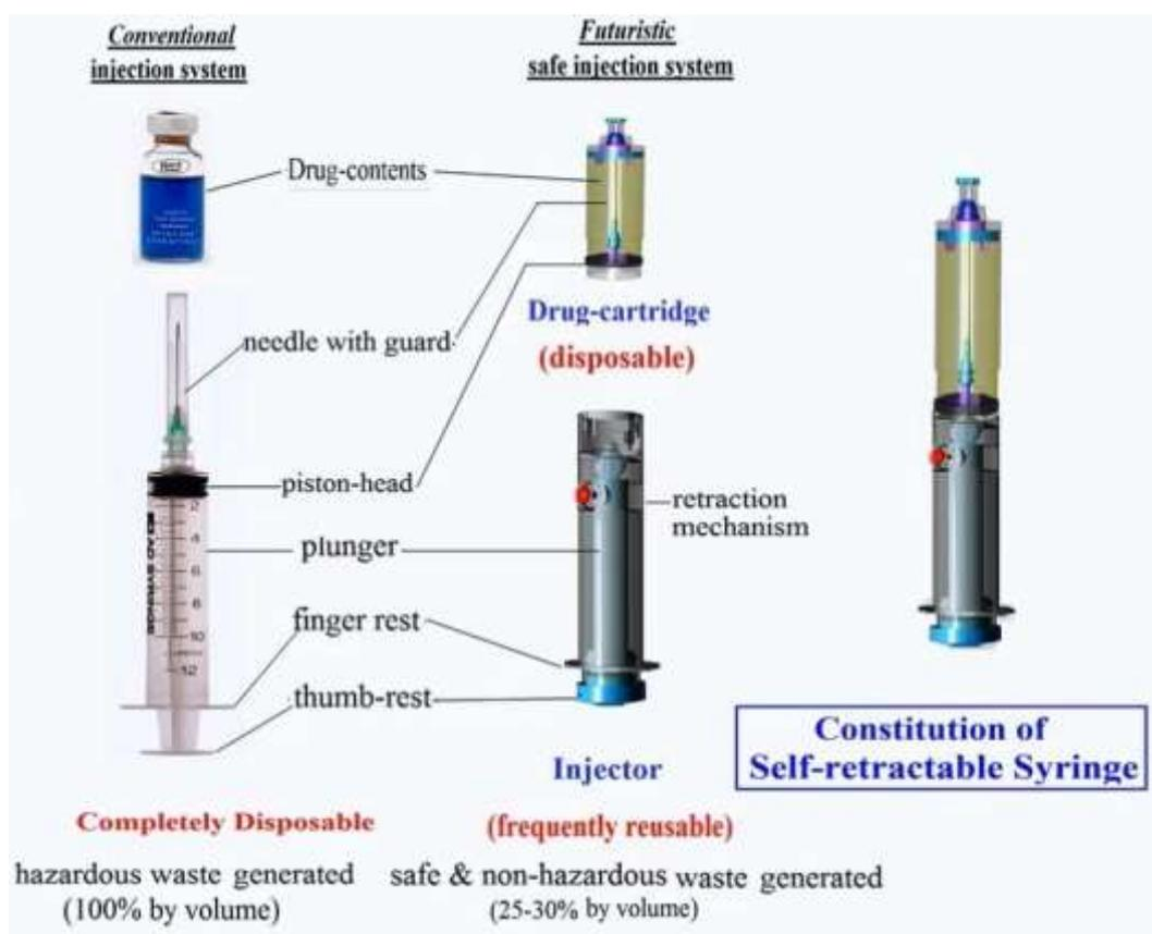
'Futuristic Safe Injection System' provides **two variants** of *reusable injectors*, multiple variants of *safely disposable drug-cartridges* and a *fluid-collector*, each one functioning distinctly depending upon various operational situations and requirements.
