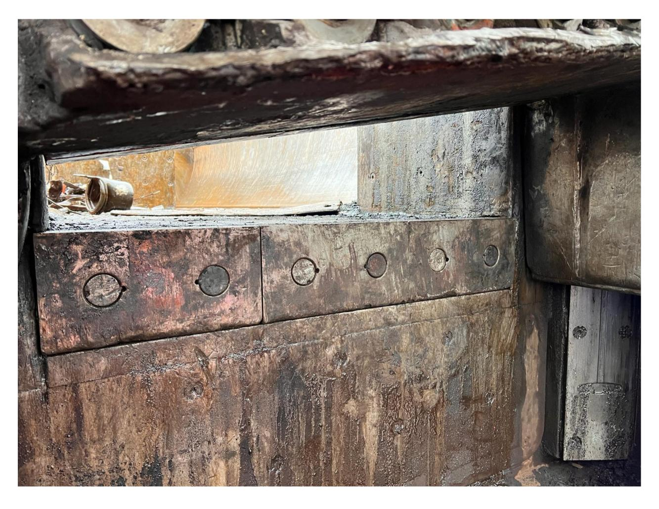
An edge view after 25.000 cuts at Heavy Metal Scrap. Total knife is serving roughly 100.000 cuts at this customer operation.
