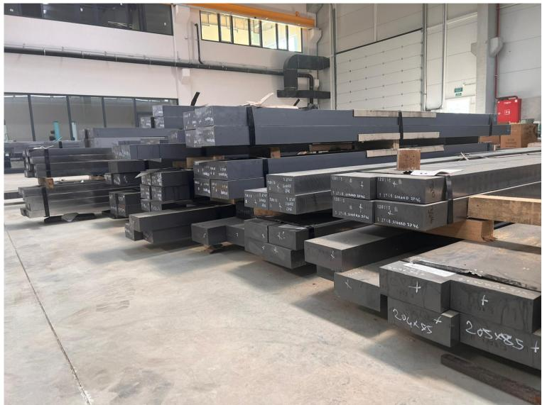
Forged and rolled flat bars in stock with different knife dimensions.
