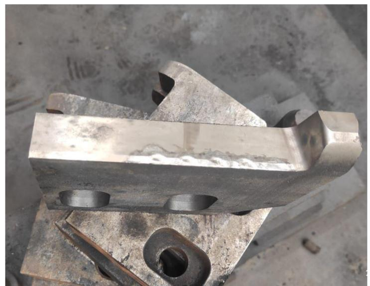
Deformation after 13.500ton production. Ø14-Ø16 rebar, cold cutting after quenching box, temperature 350°C
