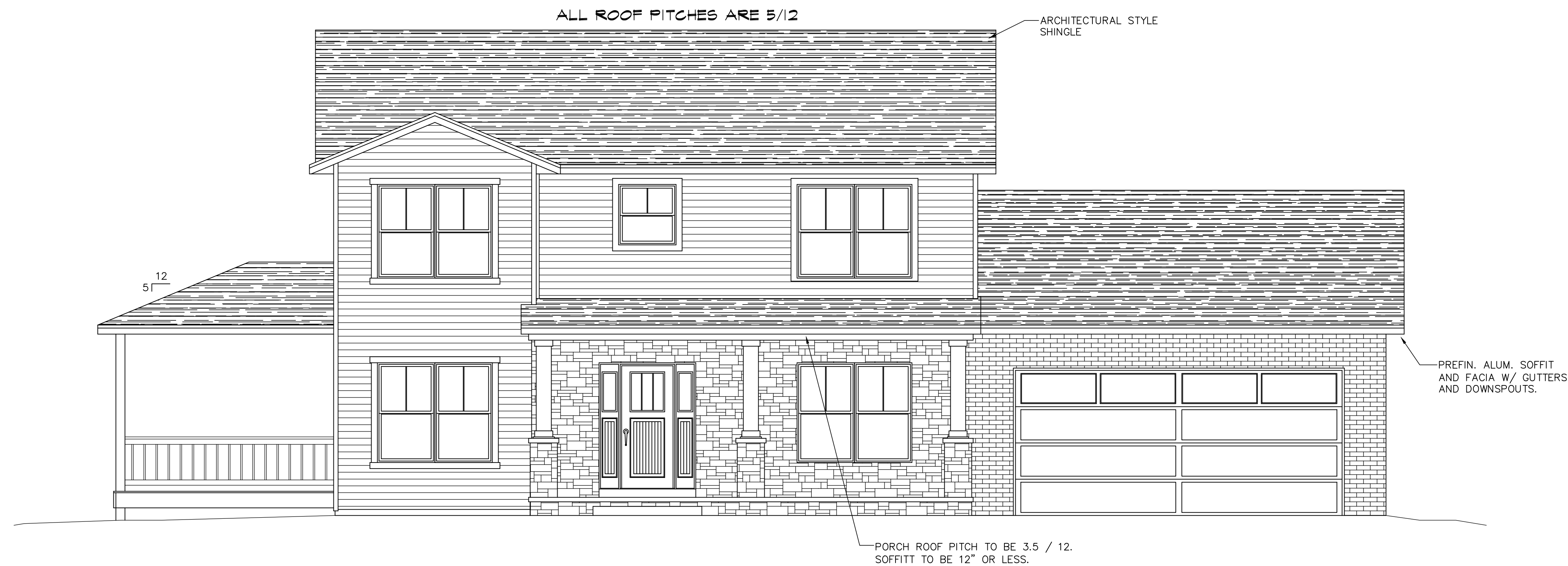
Front Elevation SCALE: 1/4" = 1'-0" 0' 4' 8' 12'
