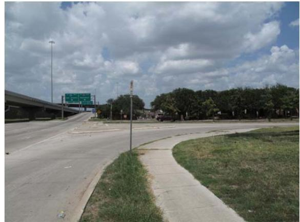
East sidewalk of US 59 northbound frontage road crossing Runnels Street – note the slip lane designed for high speed turns at the crosswalk
