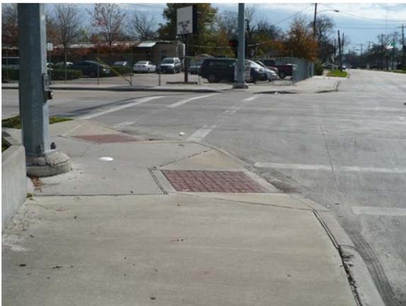
The intersection of Lyons Avenue and Gregg Street shows good sidewalk design. Although the striping is worn, crosswalks, ped signals and buttons, and ramps are provided in all directions. The sidewalks are wide and smooth.
