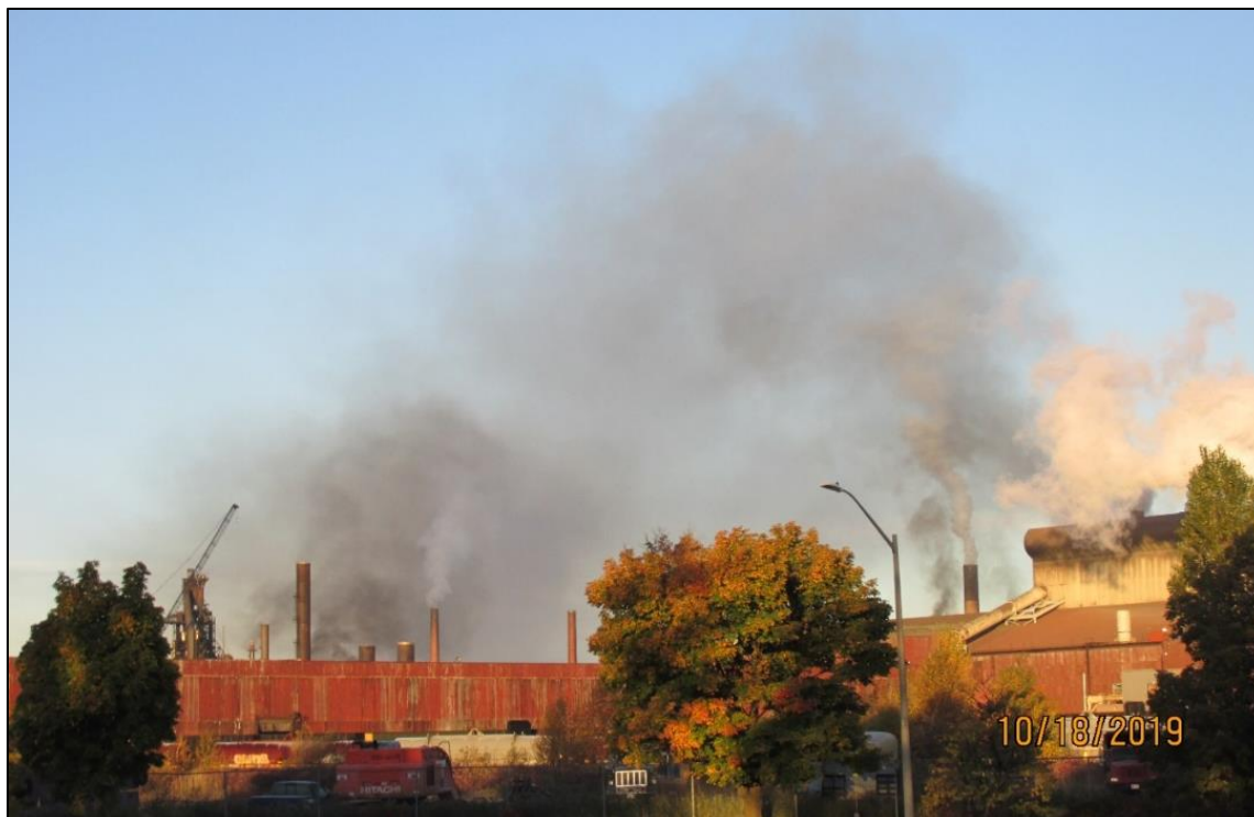
Photo 8: Particulate emissions from coke oven battery stacks (7,8,9) and flares stacks @8:26 am
