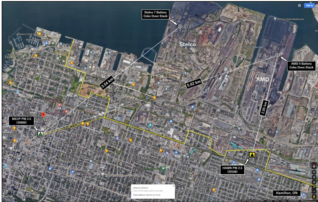
Photo 17: Distance of MECP and HAMN PM 2.5 monitors to AMD and Stelco’s closest COB stack
