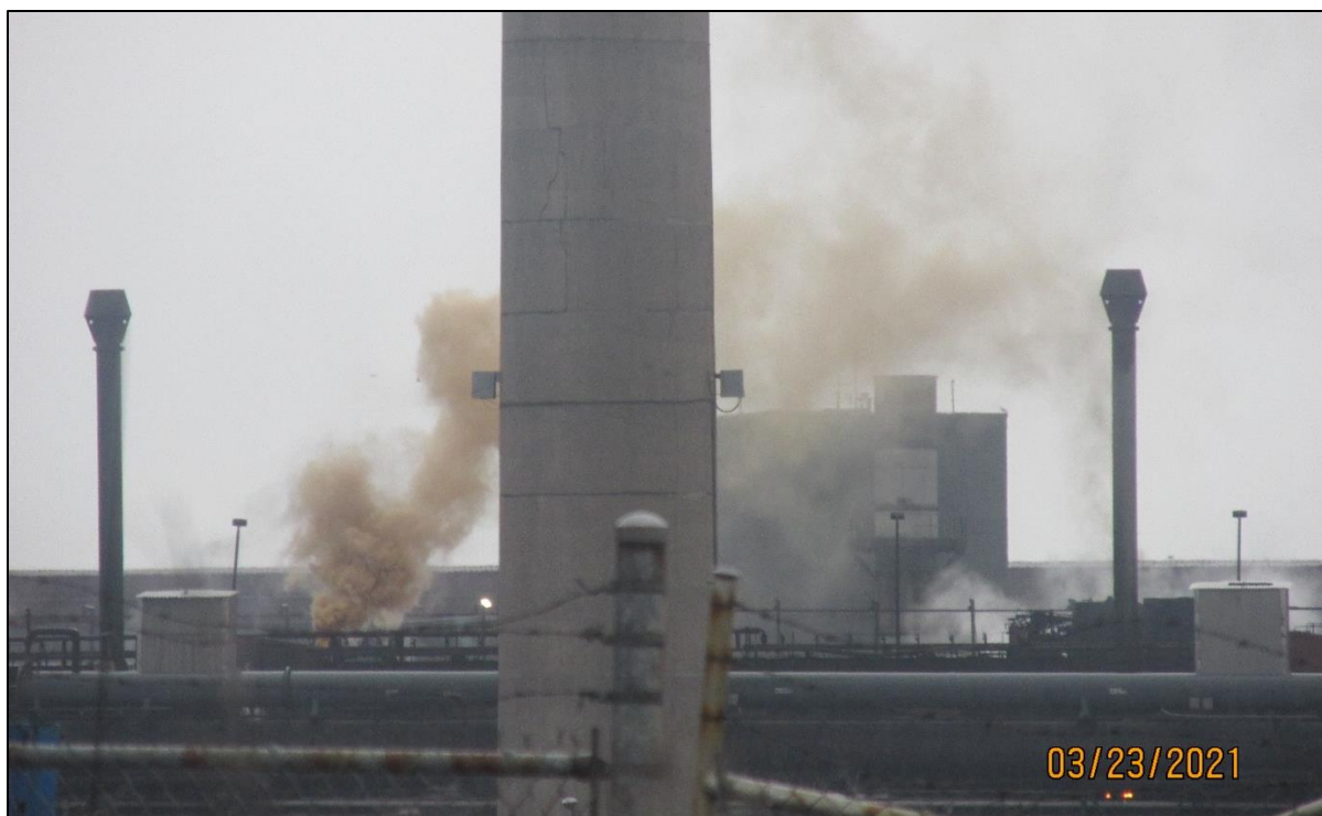
Photo 16: Raw coking gas being released from 8 Battery standpipe.
