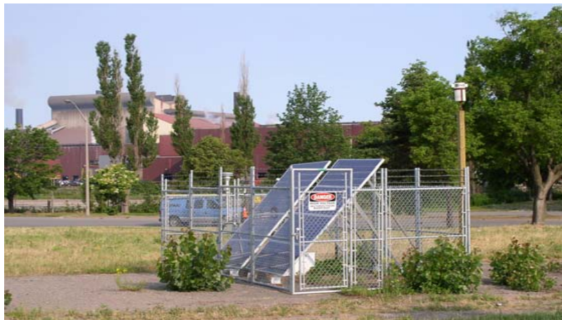
Figure A7: 71104 – Cathcart monitoring station with off-grid solar system
