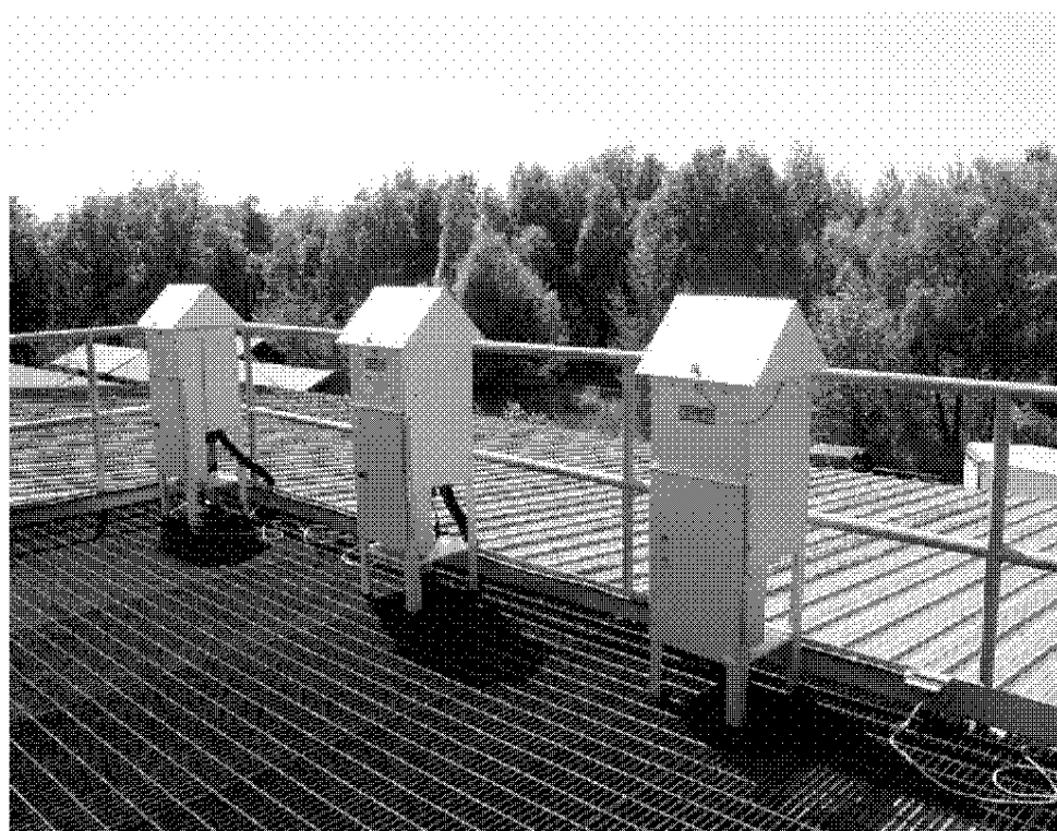
Figure 2: TSP, PAHs samplers, and VOCs inlet for the co-located audit at the Wallace Terrace station in Sault Ste. Marie.
