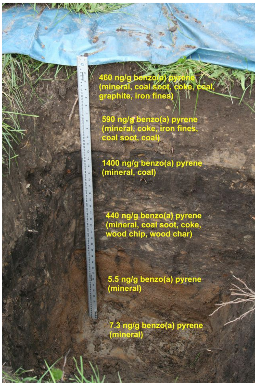
Photo 3: Soil Pit B. Benzo(a)pyrene concentrations and components that comprised more than 10% of the material in each layer/horizon are superimposed on the photograph to correspond to the layer/horizon sampled. (Photo by M. Dixon, 18 September 2013)
