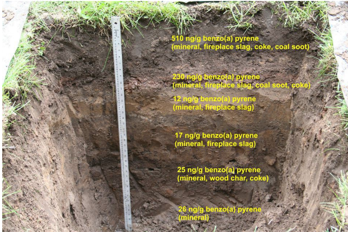
Photo 5: Soil Pit D. Benzo(a)pyrene concentrations and components that comprised more than 10% of the material in each layer/horizon are superimposed on the photograph to correspond to the layer/horizon sampled. (Photo by M. Dixon, 18 September 2013)
