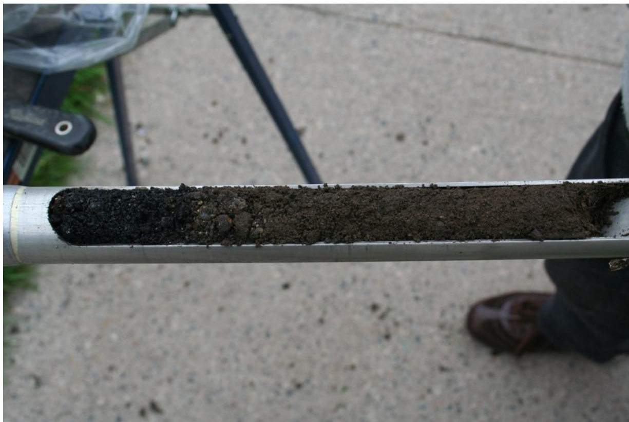
Photo 1: Soil core collected at Site 207. The surface layer of loam soil is shown on the right side, with a layer of nodules and black gritty material, sampled at depth, on the left side. (Photo by S.21 , 19 September, 2014 )
