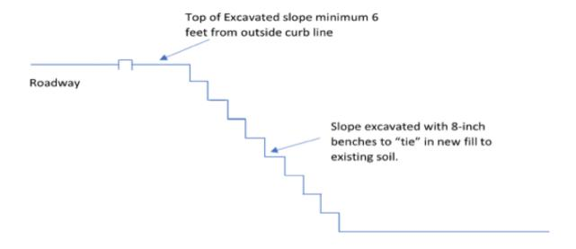
d. Structural fill materials should be low plasticity soil (Plasticity Index less than 30), free of non-soil materials and rock fragments larger than 3 inches in any one dimension. Organic and/or debris-laden material is not suitable for use as structural fill.
