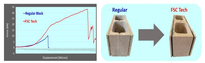
The flexural strength of Concrete Blocks is dramatically improved.
