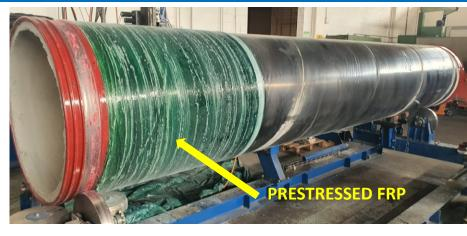
• The impermeable barrier created by the FRP and the resin eliminates the need for a cement rich, and brittle, exterior mortar coating for protecting the steel prestressing and the steel cylinder.
