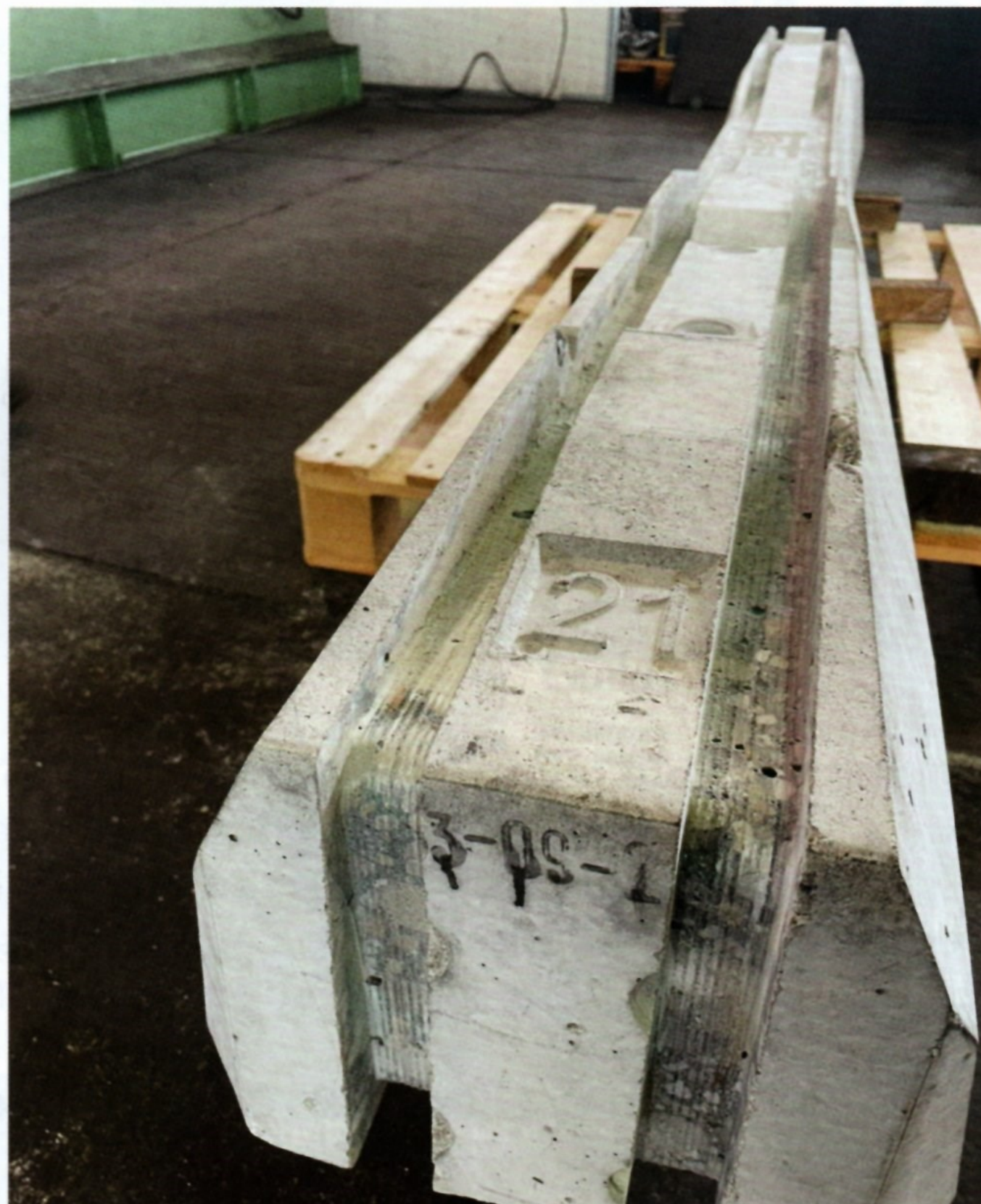
LEFT: Figure 1 – sleeper with grooves for wrapping.
