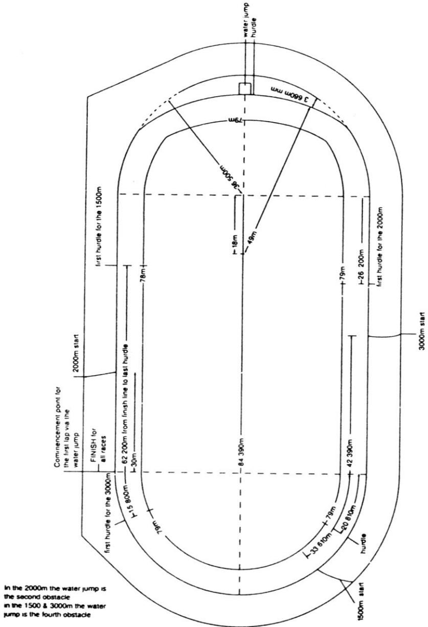
**NOTE:** This diagram is an illustration of the approximate location of starting lines and barrier locations based on an inside water jump. The specific locations will change depending on the given track layout, particularly for an outside water jump.
