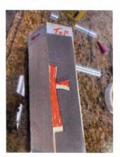
Mark the top of the project and the direction of rotation of the lathe to ensure that the tape gets tighter as it turns. Then draw the shape of the cross that you want in the center of the project.
