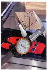
As pictured on the left, the thickness of the board needs to be as close to the width of the cut as possible.
