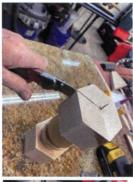
Remove the project from the lathe. Remove the tape from both ends. Using a putty or shop knife, separate the three pieces that were glued together with CA glue.
