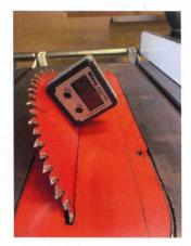
Accuracy is the key to having a successful project. This project will be 3-sided; therefore, you will need to have your saw blade set exactly to 30 degrees so that you can build 60-degree diamonds.
