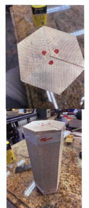
Glue these pieces together using CA glue. Mark the three pieces on the inside corners for reference.
