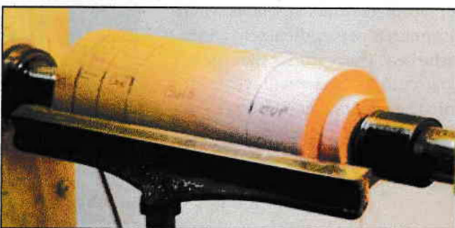
14 Mark the bottom of the cup, bottom of the bulb, bottom of small base, and bottom of large base.
