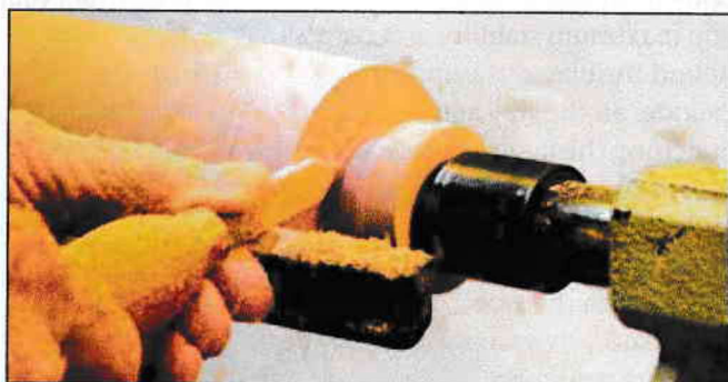
14 Mark the bottom of the cup, bottom of the bulb, bottom of small base, and bottom of large base.
