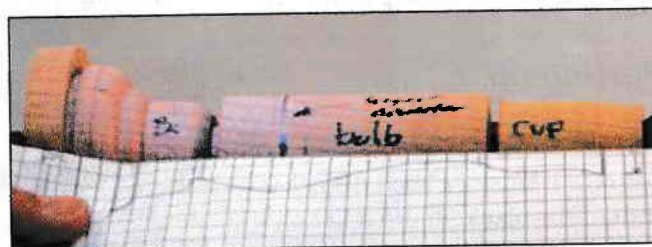
17 Shape the elements using the spindle gouge, always cutting from large diameter down to smaller diameters.
