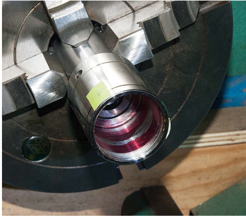
A few more passes. Small amount of dye remaining on front machined area, no dye on rear machined area.
