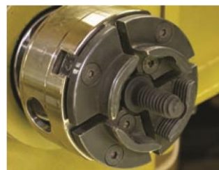
Screw chuck attached in a talon chuck showing safety power is required, talon chuck. slots and pin in jaws. using a faceplate is Open-back talon chuck with key.
