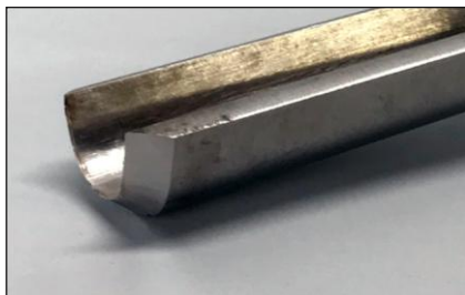
Spindle roughing gouge
