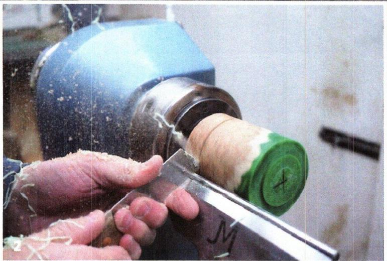
◀ **3** Use a 19mm skewed negative rake scraper to reduce the overall diameter of the lid by 10mm.
