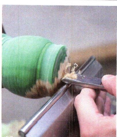
**19** In this picture you can see the lid before sanding, how the base curves in to meet the lid and the extra material at the base of the box that was referred to in Step 15.
