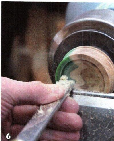
**7** Use a 25mm round-nosed negative rake scraper to refine the inside of the box surface prior to sanding.
