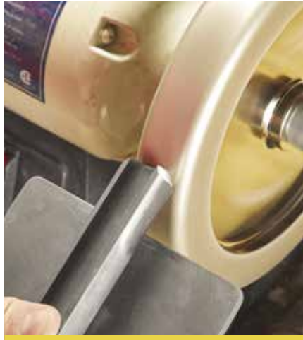
▲ An SRG can also be sharpened with the adjustable tool rest and is the safest way to sharpen an SRG with a CBN wheel.
