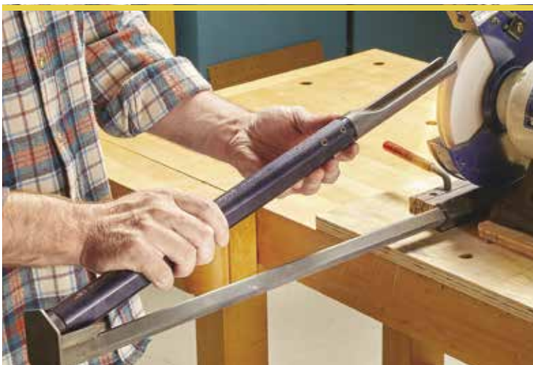
▲ Adjust the V-cradle out until the angle of the tool bevel matches the profile of the wheel. Then, lock it in place and turn the grinder on. Rest the butt of the tool in the cradle and rotate the cutting edge on the wheel to sharpen it.
