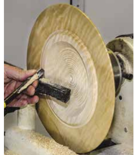
Hollowing. Work back towards the rim, finishing the interior in sections at a time to minimize any movement in the rim.
