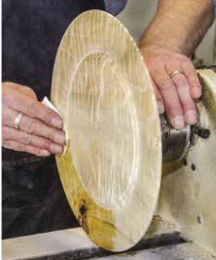
Finishing the Rim. Sand, seal, and finish the rim. It's best to do this before hollowing, in case the rim moves afterward.
