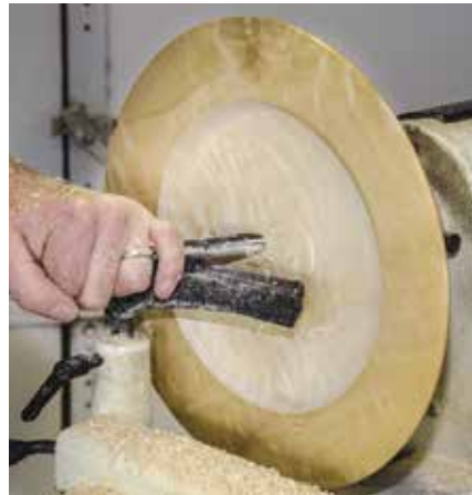
Final Cuts. Make smooth push cuts from the outside towards the center, being careful not to break through the recess.
