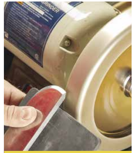
▲ Negative rake scrapers are sharpened long bevel (bottom) first, then the shorter second bevel for a 70° edge.
