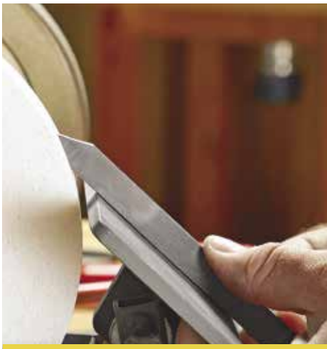
▲ Match the angle of the tool rest so the parting tool is resting on the wheel. Then, sharpen both sides of the parting tool keeping the end square.
