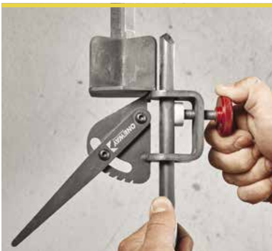
▲ Setting the protrusion is what will give consistent results with the Vari-Grind jig. I use the V-cradle as a gauge to get the same setup every time.
