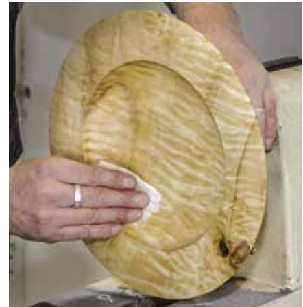
Finishing. Once you've reached the desired shape, sand, seal, and oil the platter, then let it cure before using it.
