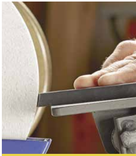
▲ Traditional scrapers are easiest to sharpen upside-down. The tool rest is angled down to drag a burr off the top (cutting) side.
