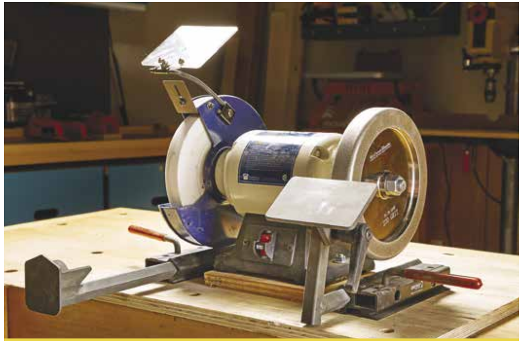
▲ A basic turning sharpening setup is shown here. The Oneway Wolverine system includes a V-cradle and a platform. Both of which slide into receivers mounted below the wheel to adjust for different tools and bevel angles.
