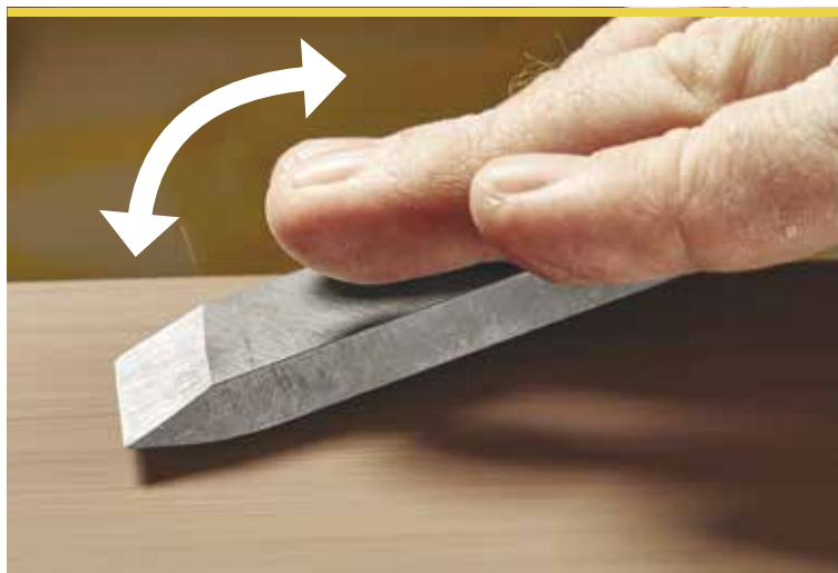
▲ The first thing I do on a skew chisel is to round over the bevel shoulders. Use a belt sander. Start with the bevel “line” on the belt and raise and lower the tool handle to round over the bevel face.
