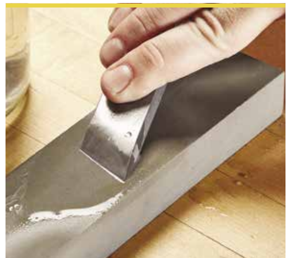
▲ For final sharpening after shaping the skew, I go to an oilstone. Then, it's just a simple matter of putting an edge on like you would a normal bench chisel.
