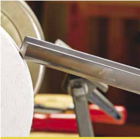
▲ Adjust the V-cradle until the bevel on the spindle roughing gouge matches the curvature of the grinding wheel.
