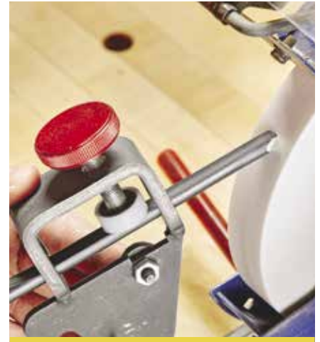
▲ The spindle gouge can easily be sharpened using the Vari-Grind jig. The tool is rocked back and forth to sharpen the entire bevel.
