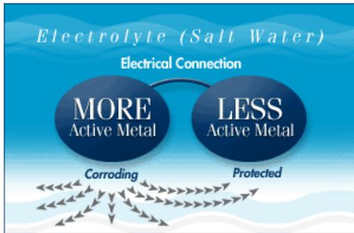
All metals immersed in an electrolyte (sea water for example) produce an electrical voltage. When two dissimilar metals are in contact (electrically connected) they produce a galvanic cell (like a battery), with the less noble metal (a bronze propeller for example) forming the anode and the more noble metal (stainless steel shaft) forming the cathode.
