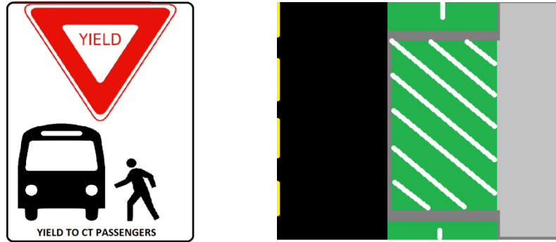
*Examples of signage and sidewalk extension, ramps and markings in bus zones
